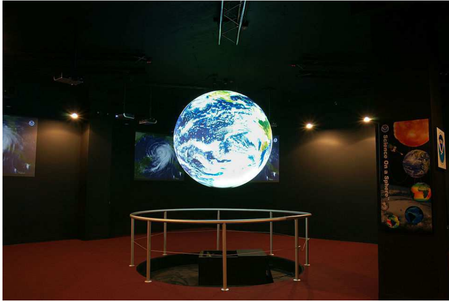
Figure 1: The setup of the original SoS system projecting the content onto a spherical projection globe using 4 projectors.
