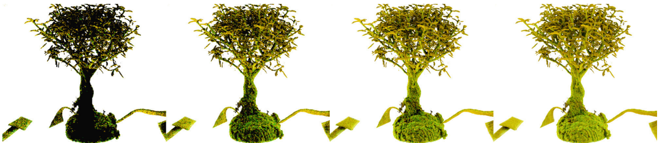
Figure 1: Progressive refinement of a rendering of the bonsai dataset. The resolution of the dataset was 512 \times 512 \times 182 , and the resolution of the internal frame buffers was 512 \times 512 . At 20 frames per second the first image appeared on the screen in a fraction of a second, showing a recognizable shape. The last and most accurate image took 10 seconds to generate.
