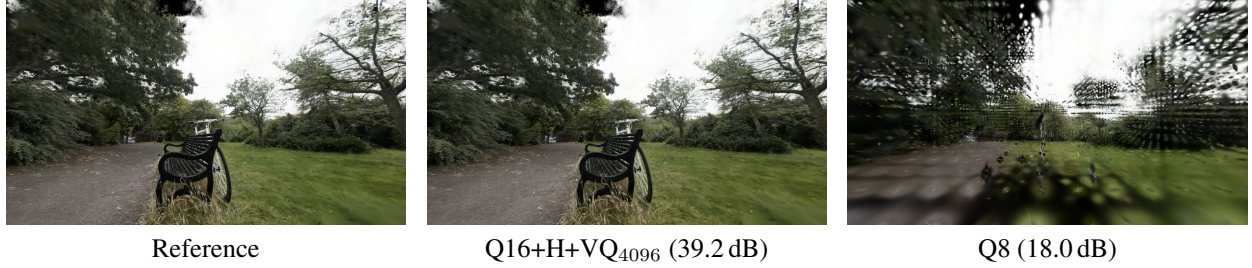
Figure 1: Visual comparison on the bicycle scene (0° camera angle): reference render, best configuration Q16+H+VQ 4096 , and worst configuration Q8 which introduces severe quantization artifacts.
