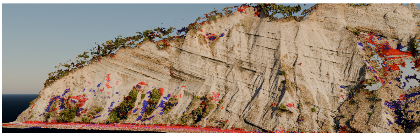
Figure 1: A render of a UAV point cloud with M3C2 distances overlaid in regions of significant change.
