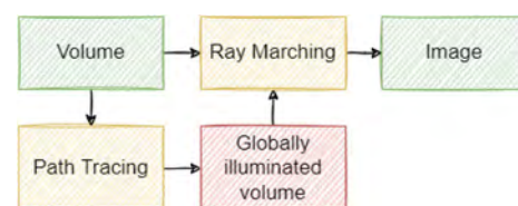
Fig. 2 An overview of the caching technique for combined volume and surface rendering
