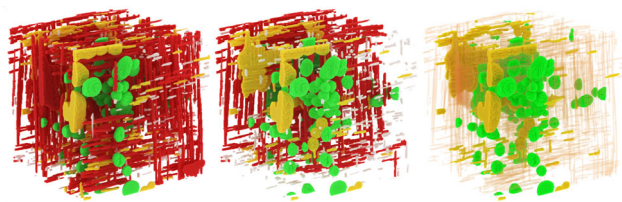
Fig. 8 Use case with pores. From left to right: (1) colorization by roundness (needle-shaped pores are red), (2) the same as (1) but with 50 % of the needle-shaped pores hidden by depth, and (3) the same as (2) but with a higher transparency of needle-shaped pores to emphasize the round ones
